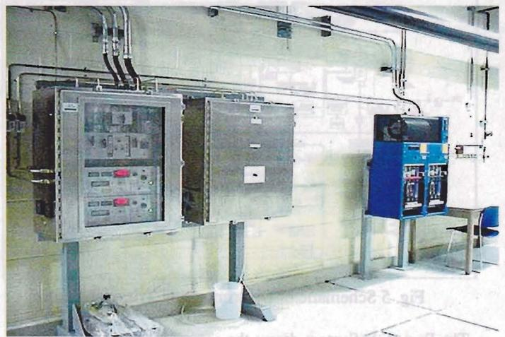
Fig. 10 The Discriminating Tritium Monitor with C-14 Sampler
