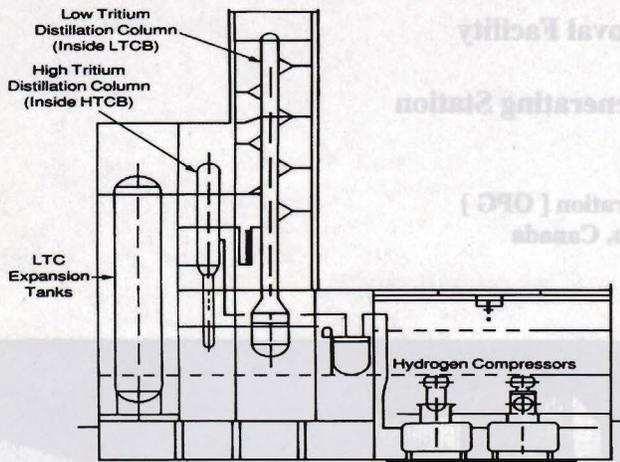
Fig. 3 The Heavy Water Management section of the Tritium Removal Facility
