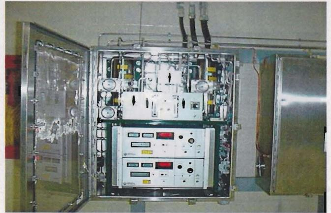
Fig. 7 View of Ion Chambers and Data Display
