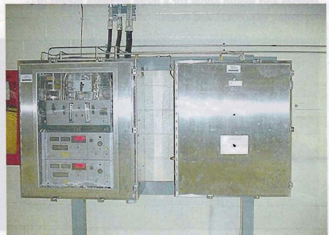
Fig. 4 The Discriminating Tritium Monitor with Dryer
