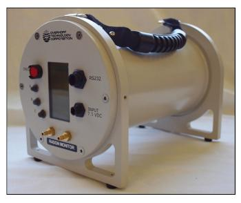
Particularly useful as a real-time radon monitor for those involved in radon mitigation since the fast, sensitive, real-time measurement gives an immediate indication of any mitigation efforts. Mitigation of radon concentrations can be as simple as a change in ventilation flow or a more complex effort such as installing a vapor barrier.
