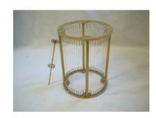
Wire-Grid Chamber Design, reduces tritium contamination by up to 1000x
