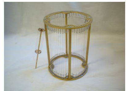
Wire-Grid Chamber Design, reduces tritium contamination by up to 1000x
