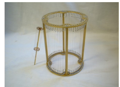
Wire-Grid Chamber Design, reduces tritium contamination by up to 1000x
