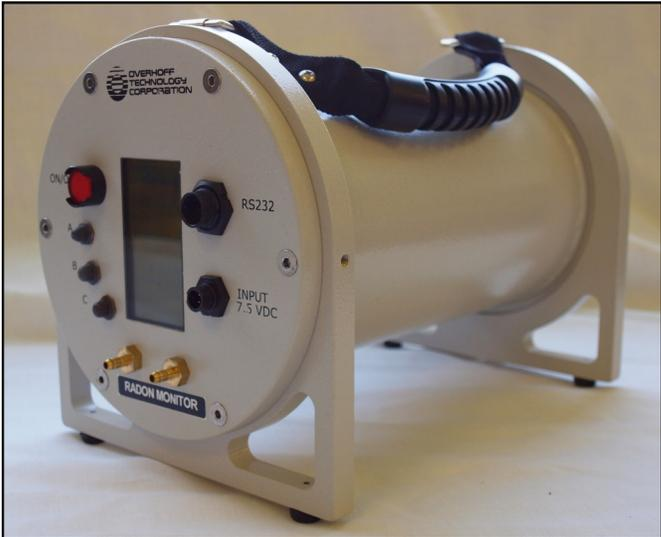
The radon monitor can log 40,000 data points to accurately establish the daily variation in radon concentrations. The radon monitor's internal rechargeable battery can operate the monitor for 24 hours. By using the AC/DC adapter the monitoring time can be extended indefinitely which allows for logging the variations in radon concentrations due to the environmental effects of changes in barometric pressure and rainfall.
