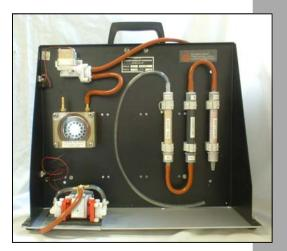
New Product from Overhoff Technology Corporation enables precise measurement of tritium in the presence of noble and other radioactive gases. The separator extracts the tritium oxide component of a continuous air sample, which may also contain Xenon, Krypton-85, Carbon 14, or other radioactive gases. The tritium only output airflow is then connected to an external tritium monitor, for an accurate tritium only measurement.
